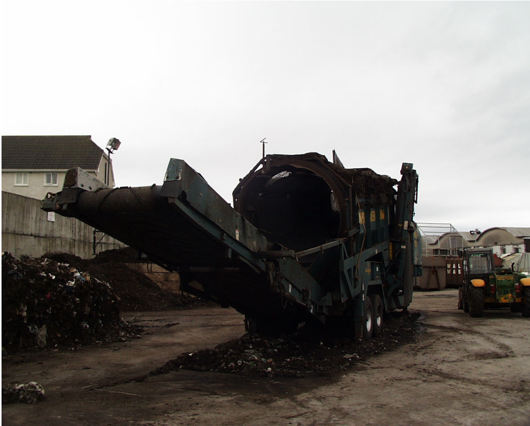
A Trommel as seen at Sandy Road Composting Facility
