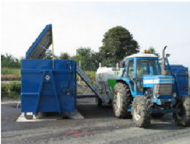
Fig. 1. Loading an in-vessel digester at Dungarvan.
